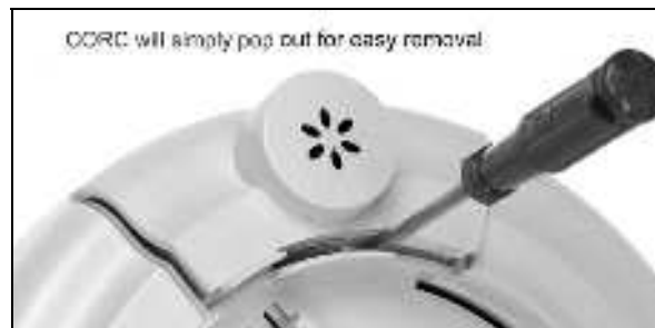
Figure 3-9. Removing the CORC from the Sensor Base
