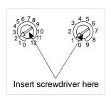
**Example:** device address 21, set TENS rotary switch to 2 and set the ONES rotary switch to 1.
