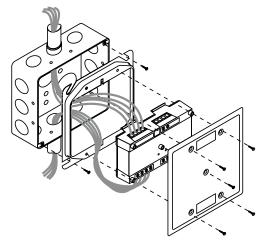
**GSA-MCC1 and GSA-MCC2:** mount the UIO motherboard inside a suitable Kidde enclosure with screws and washers provided. Plug the GSA-MCC1 or GSA-MCC2 into any available position on the motherboard and secure the module to the motherboard with the captive screws. Wiring connections are made to the terminals on the motherboard (see wiring diagram). UIO motherboard terminals are suited for #12 to #18 AWG (2.5 mm<sup>2</sup> to 0.75 mm<sup>2</sup>) wire size.
