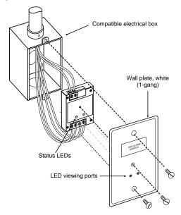
**SIGA-MCR** and **SIGA-MCRR**: mount the UIO motherboard inside a suitable EDWARDS enclosure with screws and washers provided. Plug the module into any available position on the motherboard and secure the module to the motherboard with the captive screws. Wiring connections are made to the terminals on the motherboard (see wiring diagram). UIO motherboard terminals are suited for #12 to #18 AWG (2.5 mm² to 0.75 mm²) wire size.
